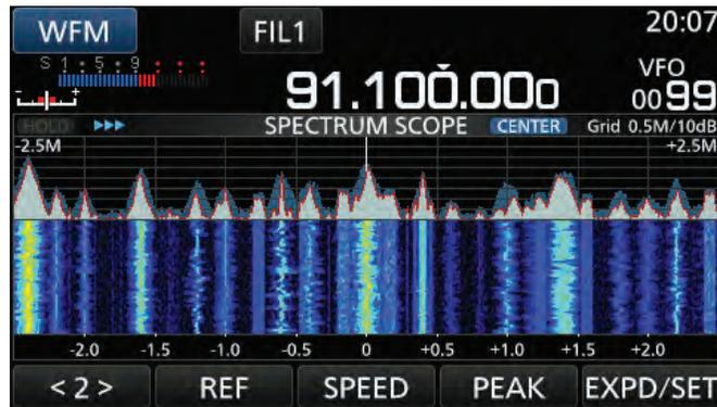
Figure 3 — Spectrum of FM broadcast signals.
