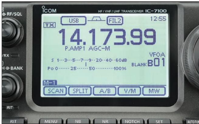
**Figure 5** — The IC-7100's screen is larger than that on the IC-706 and IC-7000. Touching various spots on the screen such as the soft keys across the bottom or the frequency display brings up menus or changes settings.
