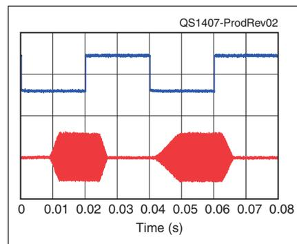
**Figure 2** — CW keying waveform for the Icom IC-7100 showing the first two dits in full break-in (QSK) mode using external keying. Equivalent keying speed is 60 WPM. The upper trace is the actual key closure; the lower trace is the RF envelope. (Note that the first key closure starts at the left edge of the figure.) Horizontal divisions are 10 ms. The transceiver was being operated at 100 W output on the 14 MHz band.
